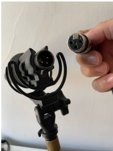
Plug in the microphone (XLR) cable into the back of the microphone
